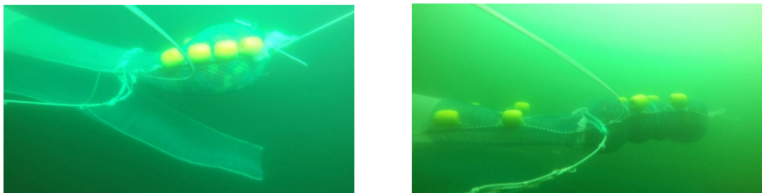
Figure 3: Left: Codend in pear shape without ring reinforcements. Right: Codend in cylindrical shape with four ring reinforcements.
